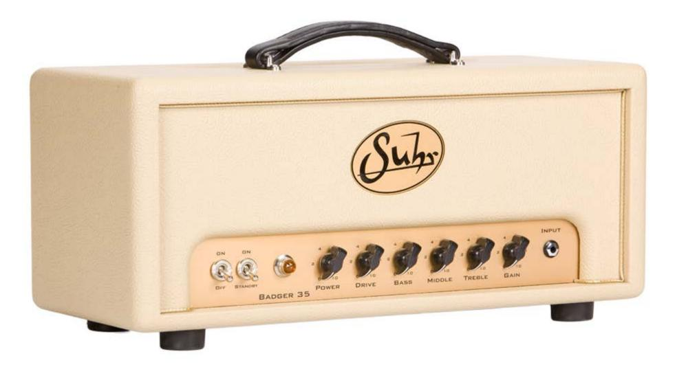
ON/Standby: With the Power switch in the OFF position and the Standby switch in the STANDBY position, flip the power switch to ON. Wait 60 seconds, then flip the Standby switch to the ON position. This will prolong tube life. To power down, simply switch the power switch to the OFF position.
